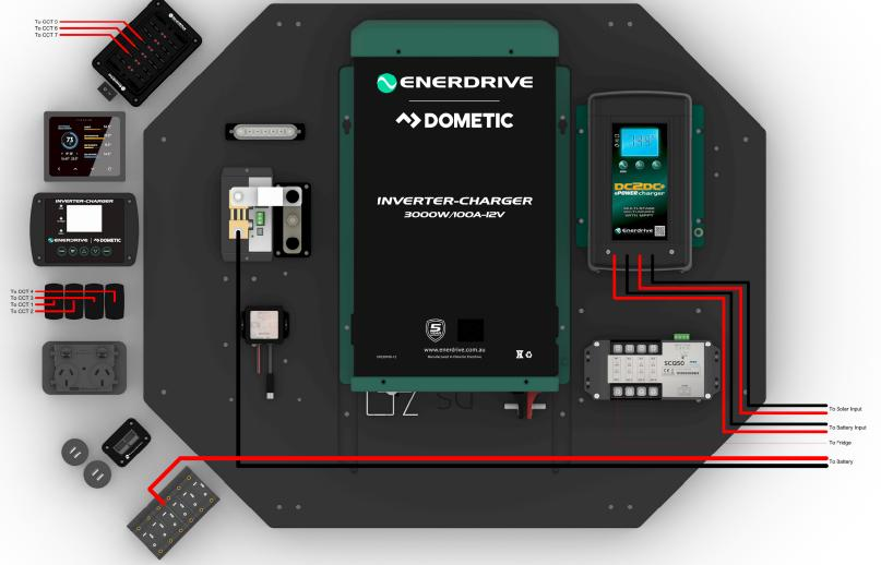
NOTES: CABLE SIZES: PROJECT: VOYAGER ALL EXTERNAL CABLE SIZES 95mm2 1mm2 PASSENGER WIRING DIAGRAM PROVIDED ARE A GUIDE ONLY. **INSTALLER** Pico Cable LOAD REQUIREMENTS MAY VARY, PLEASE SIZE ACCORDINGLY. DRAWN BY: DATE: 27/07/23 M. MCDOUGALL Comms Cable IF UNSURE, REFER TO LOCAL (as required) DATE: 27/07/23 APPROVED BY: D. BALL STANDARD REGARDING CABLE SIZING FOR EXTERNAL LOADS. 4mm2 SCALE: SHEET: 1 OF 1 1:5.5
