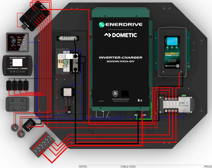
PROJECT: VOYAGER ALL EXTERNAL CABLE SIZES 95mm2 1mm2 PASSENGER WIRING DIAGRAM PROVIDED ARE A GUIDE ONLY. **ENERDRIVE** Pico Cable LOAD REQUIREMENTS MAY VARY, PLEASE SIZE ACCORDINGLY. DRAWN BY: DATE: 27/07/23 M. MCDOUGALL Comms Cable IF UNSURE, REFER TO LOCAL (as required) DATE: 27/07/23 APPROVED BY: D. BALL STANDARD REGARDING CABLE SIZING FOR EXTERNAL LOADS. 4mm2 SCALE: SHEET: 1 OF 1 1:5.5
