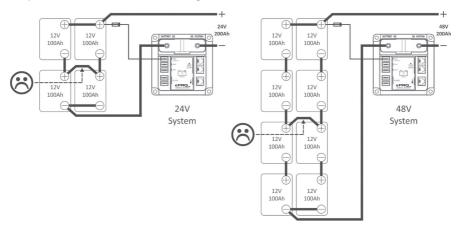
The reason for this is that through the interconnected midpoints, one bad battery in a series string can damage all other batteries if not being monitored correctly. However, when decent midpoint voltage measurement has been applied and an alarm is triggered when the voltage difference is too large, the midpoints of the series strings are allowed to be interconnected. This will result in the following connection diagrams:
