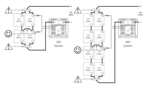
The above images are also indicating that busbars are being used to respectively join all positive and all negative battery cables. Besides this, all positive and negative battery cables that are wired to these busbars need to be of equal length. These precautions are made to avoid any imbalance between the different series strings, to ultimately improve the overall accuracy of the midpoint voltage measurement.
