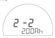
The default battery capacity value is 200Ah. This can be changed by pressing the left or right arrow keys until the desired value is reached. The standard battery capacity value is based on a discharge rate of 20 hours. When your battery capacity is rated at a different discharge rate,
