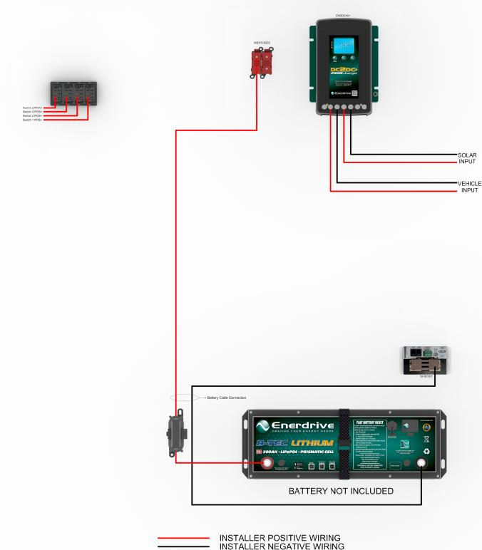
This wiring diagram is only a representation on how the wiring is done and may not fully reflect exactly how your system is wired.
