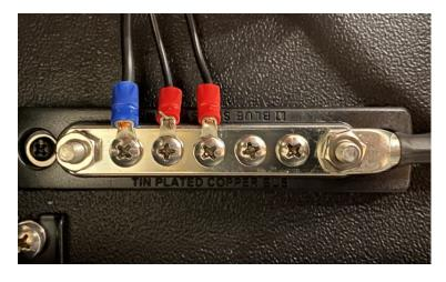
**Note:** No negative connections are to be direct to the battery or on the battery side of the shunt as this will result in incorrect reading on the Simarine system.
