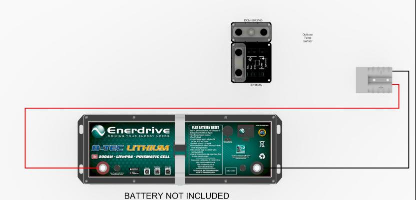
INSTALLER POSITIVE WIRINGINSTALLER NEGATIVE WIRING
