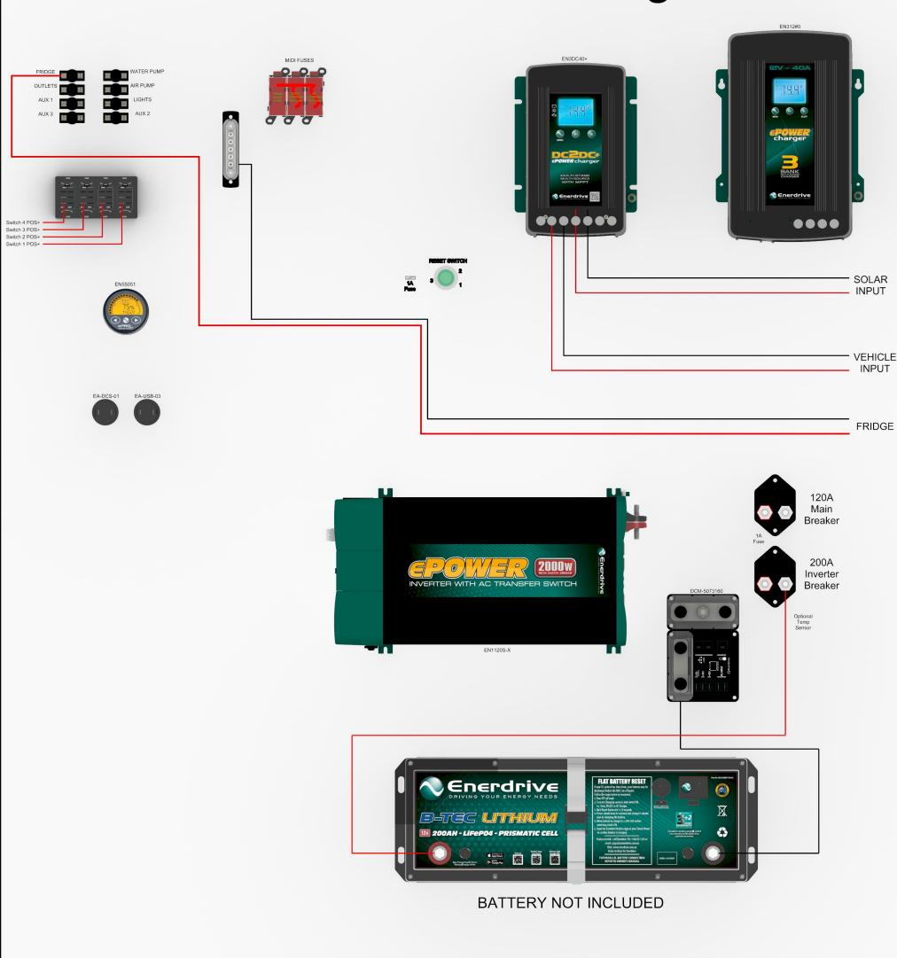
INSTALLER POSITIVE WIRING INSTALLER NEGATIVE WIRING
