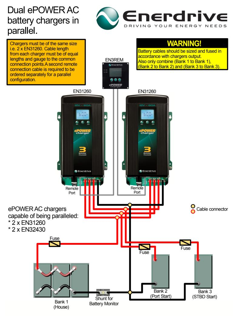
NOTE: Enerdrive Provides this drawing as a referance only and fusing and cable sizing needs to meet local requirements.
