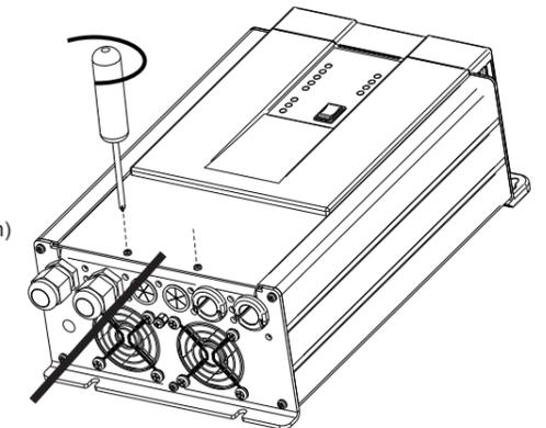
To access the connection compartment, remove the two screws indicated above and slide the red connection compartment cover downwards. Never operate this product without having the cover re-installed.
