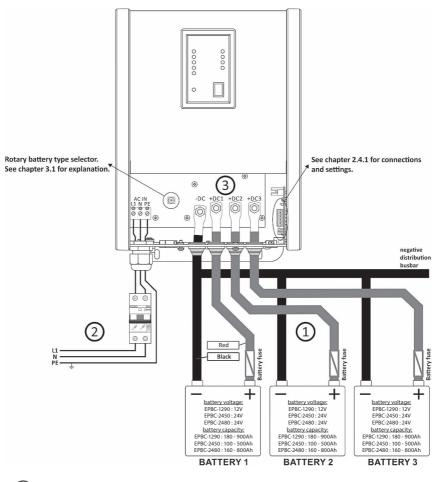
1 Please consult the following table to determine the correct battery cable and fuse size for each model. Using a smaller cable size or a longer cable will cause additional losses and may result in improperly charged batteries. Fire and burning hazards are present if the battery cables are insufficiently sized for the expected current. Battery cable lengths longer than 6 meters, are not recommended.
