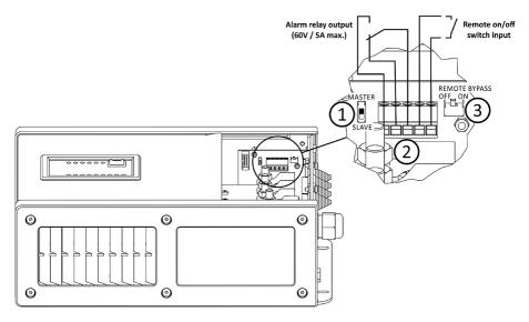
Master/slave switch position. This switch must be set to 'MASTER' when a single charger is installed. The 'SLAVE' setting is only relevant for parallel charger systems.
