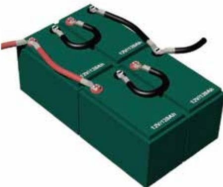
Batteries connected in series / parallel.
