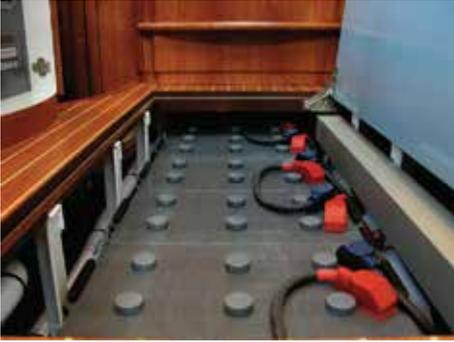
There are several ways to wire multiple batteries to achieve the correct battery voltage or capacity for a particular DC installation. Wiring multiple batteries together as one big bank, rather than having individual banks makes them more efficient and ensures maximum service life.
