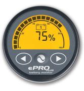
The image on the left shows the normal operating mode with the second parameter row disabled. This results in a clean display area that only shows the battery state of charge (%) and the bar graph. A perfect mode for less technical end users.
